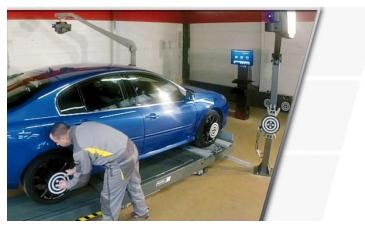
Décision Atelier for its innovation in vehicle wheel alignment and suspension testing by analyzing 3-D images.
